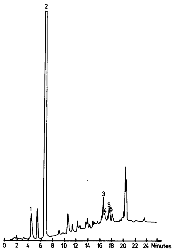
Fig. 3. Liquid chromatogram of impurities in amphetamine. Detection by UV absorption at 254 nm. Peaks as in Fig. 1.
